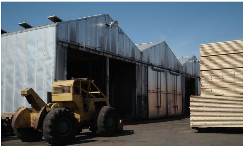
Figure 2-10 Dry Kilns Ready to be Loaded
