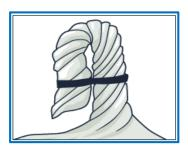
• Double-bag the folded plastic, along with the ceiling debris it contains, into pre-marked asbestos waste disposal bags. The top level of the floor plastic was put down in 100-120 square foot sections, plastic, plus wetted popcorn material on this square footage may be quite heavy, and may be all you want to carry in a single double-bagged container. Plastic and material will need to be placed in
